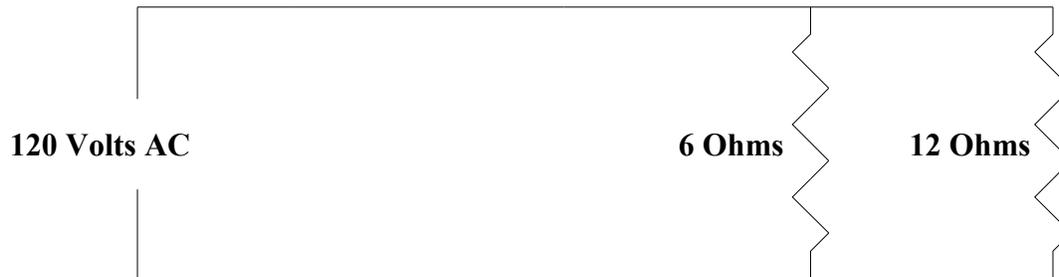
4. Based on the drawing above, what is the total circuit resistance?
